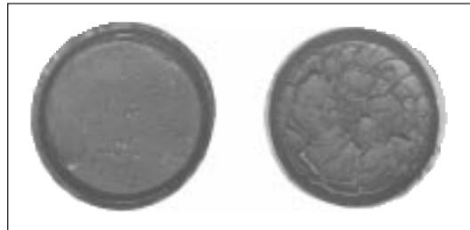
Figure 15: Cracking effect of filter cake using oil only (left) vs. PIPE-LAX and oil (right).
